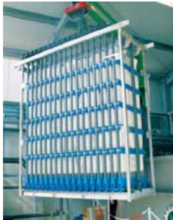
Fig.5 Typical MBR module
